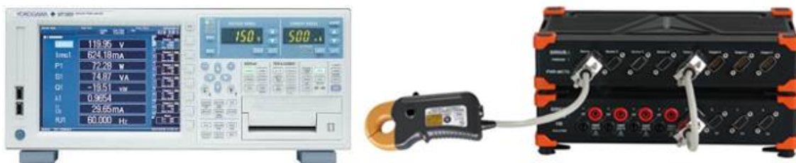
Figure 5: In-house instrumentation to measure and record electrical parameters.
