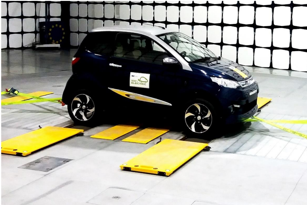
Figure 7: Aixam vehicle mounted on VeLA 9 roller benches
