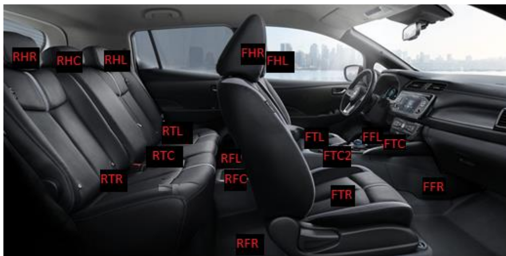
Figure 6: Identification of the measurement locations inside the vehicle.
