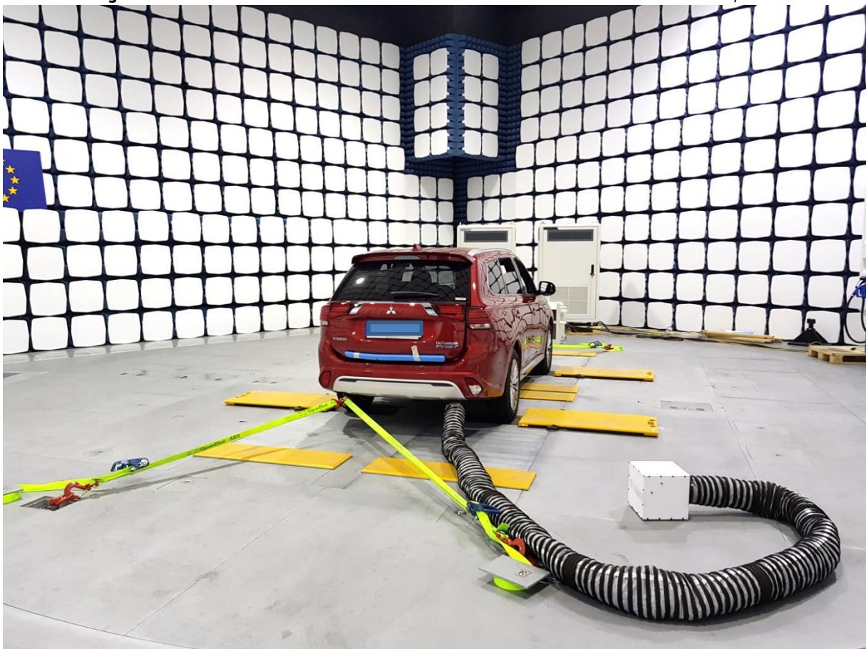
Figure 10: PHEV Mitsubishi Outlander mounted inside VeLA 9 with its exhaust extraction system
